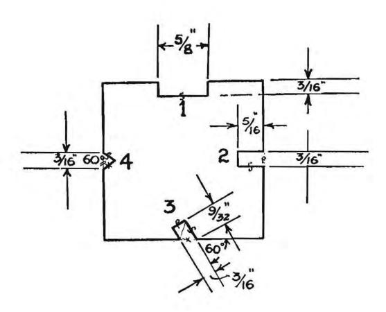
Fig. 12 Preparation board, cross section
