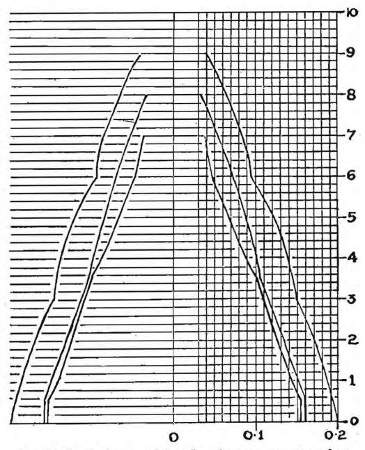
Fig. 45. Graph of tapers of three fly rods; measurements are from inner apex to centre of flat of each strip.
