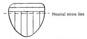
Fig. 43 Heart-shaped cross-section
