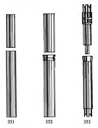
Fig. 30 (351) Plain ferrules (352) Reinforced ferrules (353) Reinforced splint-end ferrules
