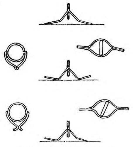
Fig. 31 Common faults in rings as received
