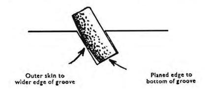
Fig. 13 Placing the strip in No. 3 groove
