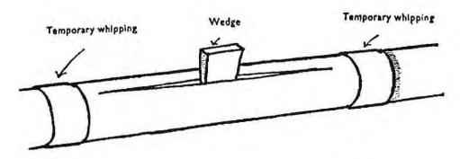
Fig. 48 Wedging open a crack for glueing
