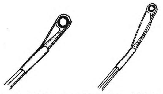
Fig. 29A Agate tip ring. Swan neck tip ring for use with High Bell's Life intermediate rings
