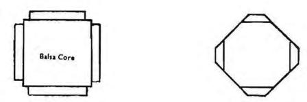
Fig. 21 (left) Building round Balsa core; first four strips in place Fig. 22 (right) Corners planed
