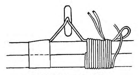
Fig. 33 Finishing a ring whipping
