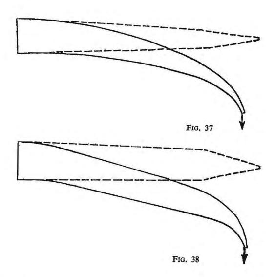
\* The greater the force used in casting, the more the rod will bend near the butt, irrespective of its taper.
