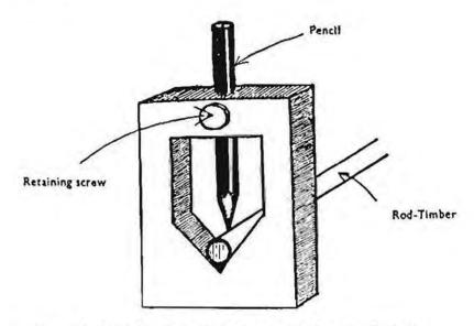
Fig. 25 Device for checking roundness of timber
