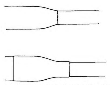
Fig. 27 (Top) After cement has set, temporary whipping removed and larger section neatly tapered
