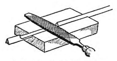
Fig. 20 Filing-block for hollow building
