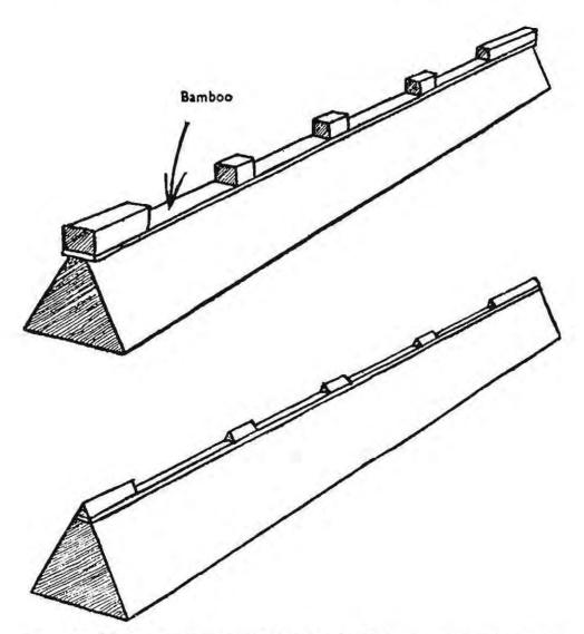
Fig. 18 Hollow building with triangular former; blocks in place Fig. 19 Blocks and bamboo planed flush with former
