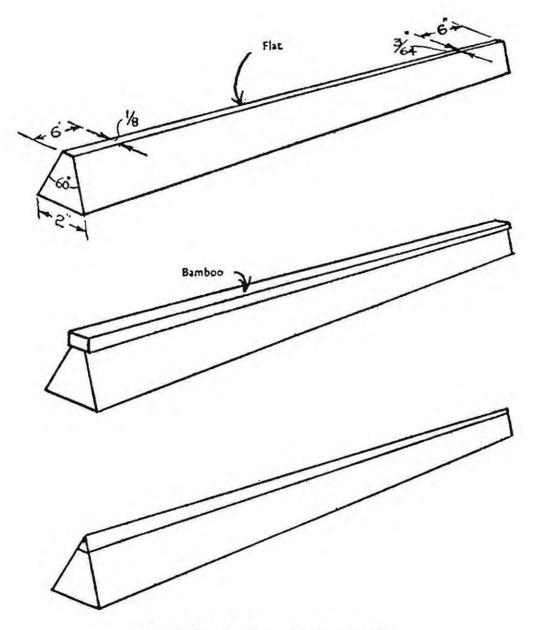
Fig. 9 (Top) Triangular former flat Fig. 10 (Middle) Bamboo glued to former Fig. 11 (Bottom) Bamboo planed flush to former
