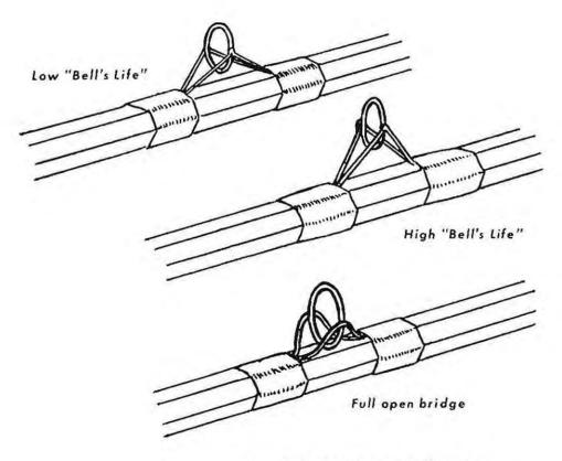
Fig. 29 Types of intermediate ring
