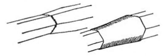
Fig. 17 Part of step taper top before and after whipping join
