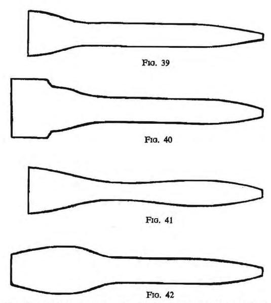
Fig. 39 Usual dry-fly taper Fig. 40 Large diameter section at butt Fig. 41 Castle Connell taper Fig. 42 Convex taper at butt
