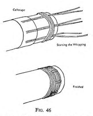
of built-up whole cane or hollow-built rods, and to heavy spinning or sea rods—in fact, to any rod where the action will not be affected—by covering with a spiral binding of hemless silk tape of the kind used for interleaving the windings of electrical transformers. The binding is laid on with the edges touching, and given several coats of varnish before the rings are whipped to the rod.
