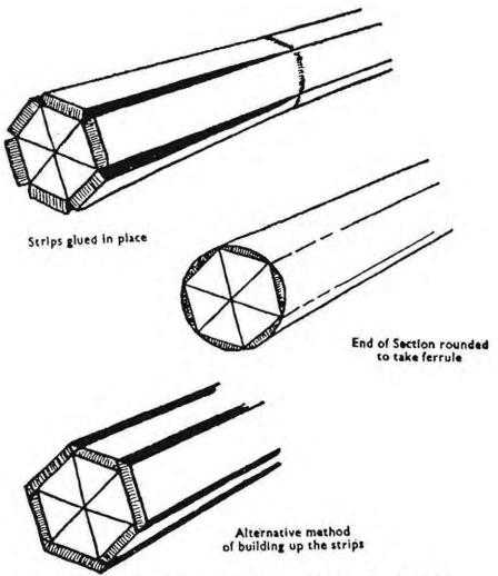
Fig. 34. Building up split cane to take the ferrules.
