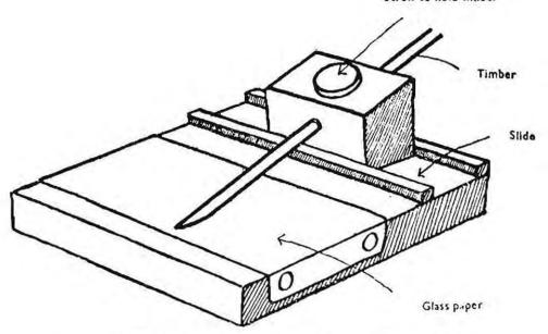
Fig. 47 Device for preparing timber for splicing
