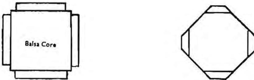
FIG. 21 (left) Building round Balsa core; first four strips in place
